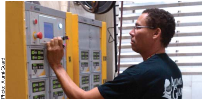
Gonzalez-Lopez adjusting a setting on Gema's Opticontrol PC based control system.
